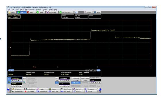
The PicoScope 9311-15 and 9311-20 generate 2.5 to 7 V steps with 60 ps rise time from built-in step recovery diodes. They are supplied with a comprehensive set of calibrated accessories to support your TDR/TDT measurements, including cables, signal dividers, adaptors, attenuator and reference load and short.
